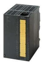
\*\*\*Spare part\*\*\* SIMATIC S7, Digital input SM 326, 8 DI; 24 V DC, NAMUR, fail-safe NAMUR input for SIMATIC S7F systems, up to Category 4 (EN 954-1)/ SIL3 (IEC61508)/PLE (ISO13849), 1x 40-pole
